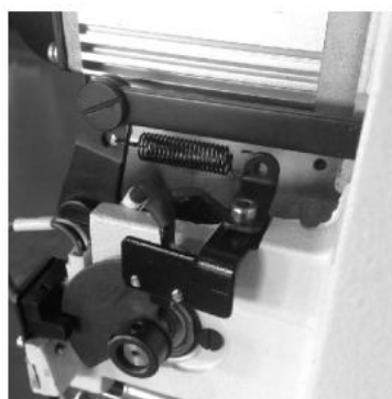
Fig.(6) After the needle protection sensor is installed (side)
